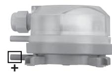
4 The pressure switches start setting should be a value which assures the function. Too low value can give undesirable activation. If it is desired to delay function until the cooker hood is working at a higher capacity, the value can be adjusted upwards. In this case, remove the protective cover from the pressure switch and adjust the knob.
