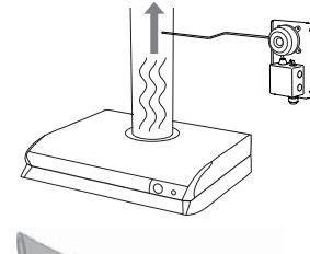
2 Drill a Ø8 mm hole in the duct and attach the pressure outlet with the arrow pointing in the direction of the air flow in the duct.
