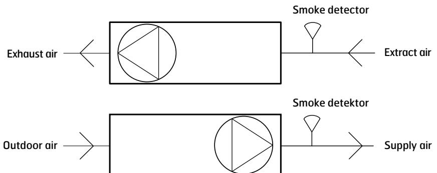
Principal drawing, connection to air handling unit
