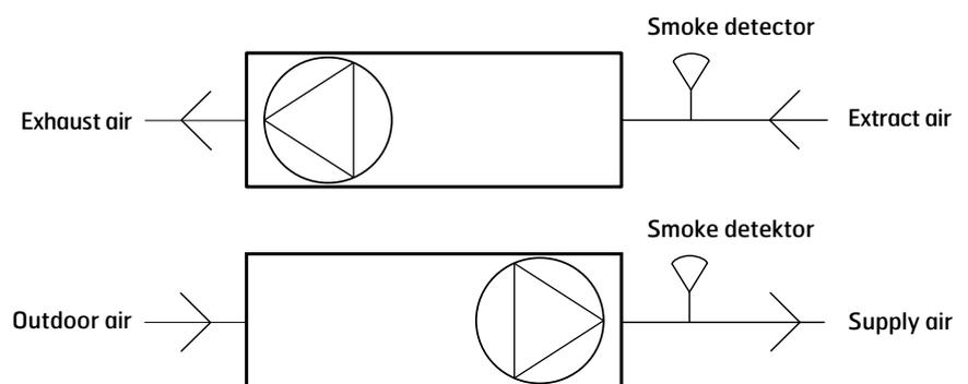
Principal drawing, connection to air handling unit
