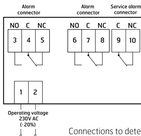
Connections to detector (normal operation / no alarm)
