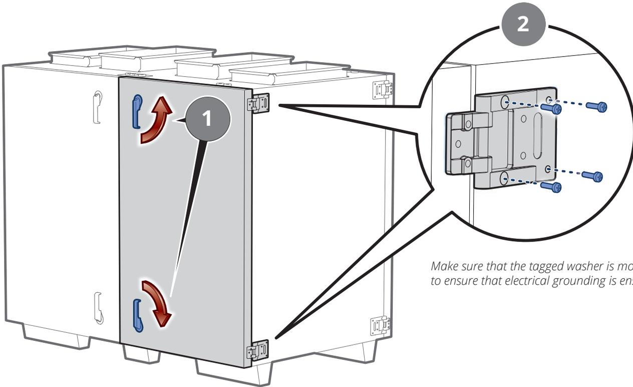
*Make sure that the tagged washer is mounted to ensure that electrical grounding is ensured.*
